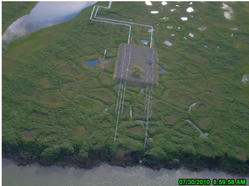
PHOTO A.10 HDD EAST, JULY 30, 2010: AERIAL VIEW OF TROUGH FROM WATER, LOOKING EAST
