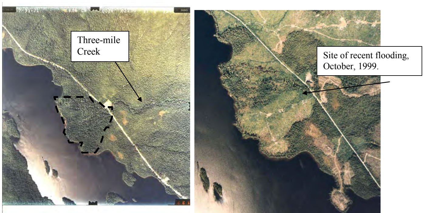
Photo 1. Three-mile Creek alluvial fan, pre-harvest 1971. Photo 2. Three-mile Creek alluvial fan, post-harvest 1991. Notice extensive ponding on the north side of the alluvial fan.
