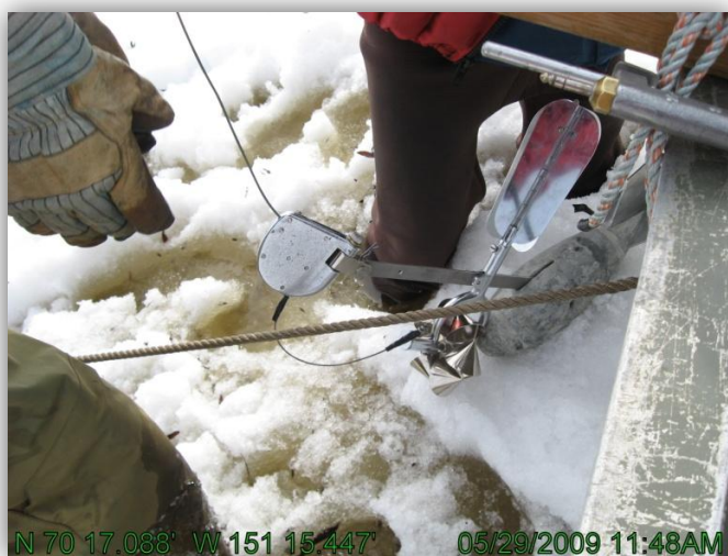
PHOTO 3.2: UBLUTUOCH RIVER BOAT DISCHARGE MEASUREMENT INSTRUMENTATION, MAY 29, 2009
