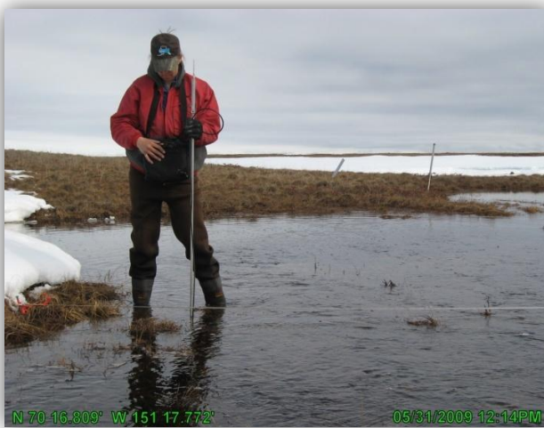
PHOTO 3.4: SMALL STREAM WADING DISCHARGE MEASUREMENT AT S4, MAY 30, 2009
