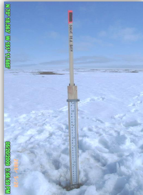
PHOTO 3.1: STAFF GAGE INSTALLED AT SITE S1, MAY 20, 2009
