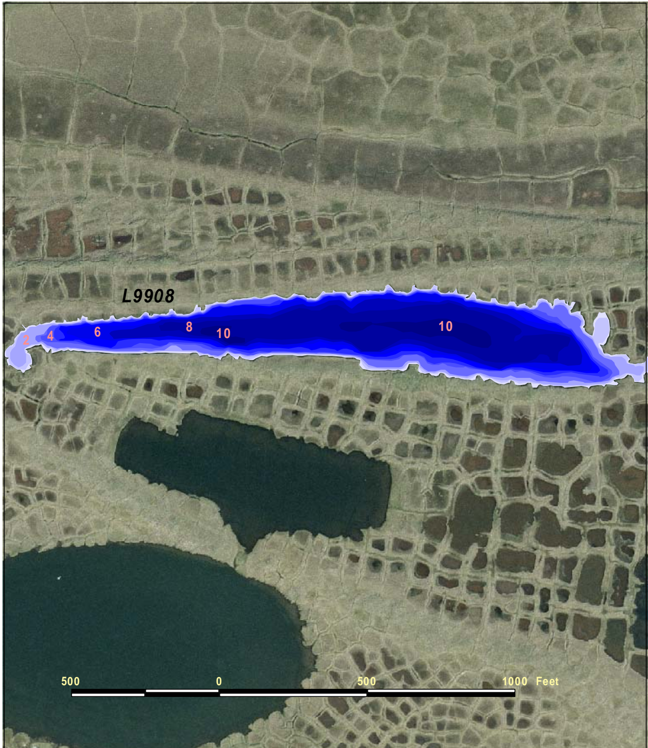
Depth contours of lake L9908 based on transects surveyed on July 29, 2006. (depths in 1 foot intervals)
