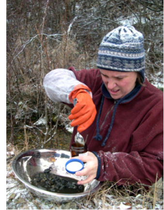
Figure 23: Soil & sediment samples were collected during the study to test for heavy metal and hydrocarbon contamination
