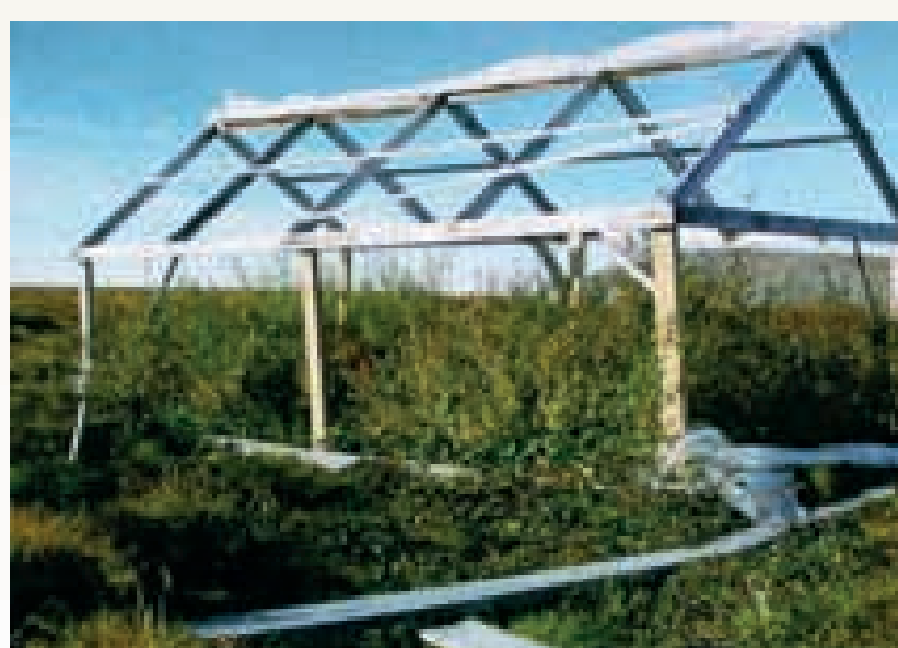
Figure 7. Experimental greenhouse with the side and top opened to show enhanced growth due to added warmth. Pre-treatment shrubs were same height as vegetation in the foreground.
