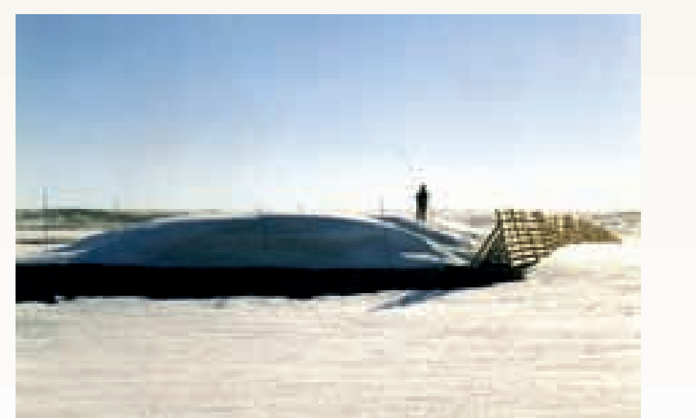
Figure 9. Winter view of snowfence experimental area showing the drift that forms behind the fence. Tall stakes are the same as striped stakes in Figure 8.
